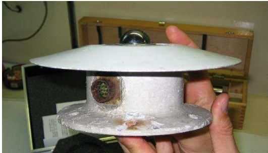
Figure 5.6: (left) Old PIR, corroded switch, no dry element, batteries empty; (right) Christopher Smarz installing the new PIR.
